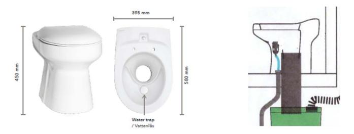
When you have measured the right place, make a hole of 210 mm to the floor. Lead the waste pipe through the hole so that about 17 cm is above the floor level.
