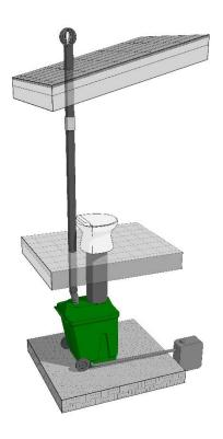
It is important to make sure that the waste pipe goes straight vertically down from the pedestal.
