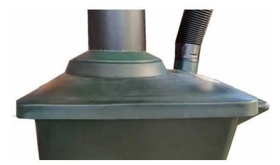
The waste shaft can come about 2-8 cm inside the Green Toilet composting unit. If the waste pipe is too long, it can be cut shorter by saw.
